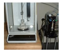
Probe tip underwater on scale during a repetitive 1 uL Differential aspiration study(standard up/down cycles, weights polled automatically when stable). This setup produced the aspiration data above.
