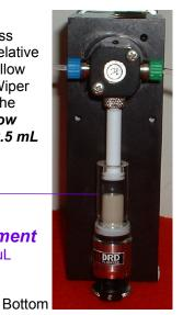
DRS 20/300 INSTALLED IN HAMILTON PSD/4 PUMP MODULE
