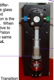
When the glass tube moves relative only to the hollow top Plunger Wiper Seal it gives the same high flow power as a 2.5 mL syringe.
