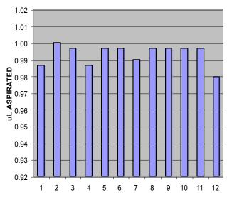
Single Displacement will blast the sample off contact-free with a standard deviation of about 0.018 uL (18 nanoliters).
