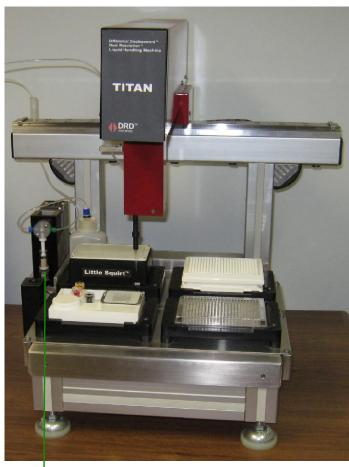
The 15/300 **Dual Resolution Syringe** is used here, but TITAN can also use other pumps like the classic Plexi or CV1dur.
