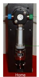
The cross-sectional area difference between the ID of the glass and the OD of the recessed spring-loaded bottom Piston is the same as a 100 uL syringe. When the glass tube moves relative to both the Plunger and the Piston simultaneously it gives the same *fine resolution as a 100 uL syringe.*
