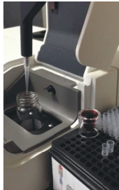
Contact-free (Blastoff /Plopoff) Differential Pipetting
